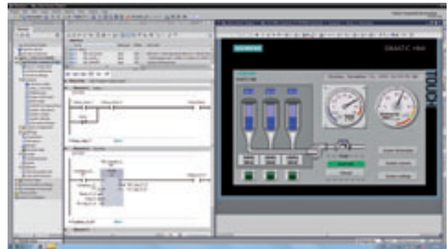
HMI editor for screen configuration of HMI Comfort Panels
